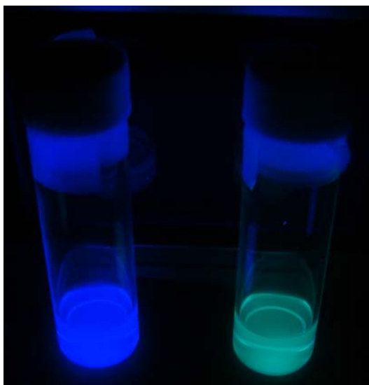
Figure 7.6. Digital images of TPPA and TPPA-Zn 2+ solutions. The solutions were irradiated with a UV lamp.
