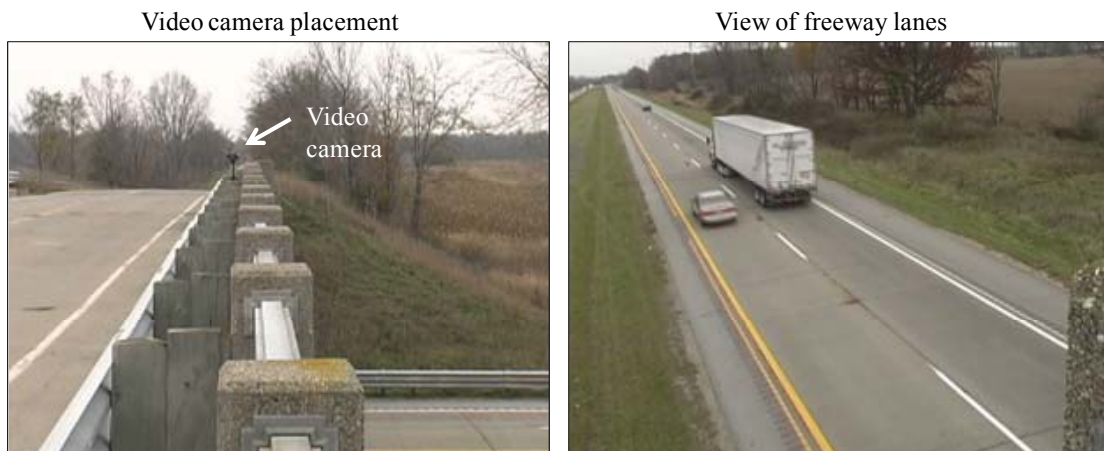
Figure 6. Typical video camera setup on sites west of Lansing
