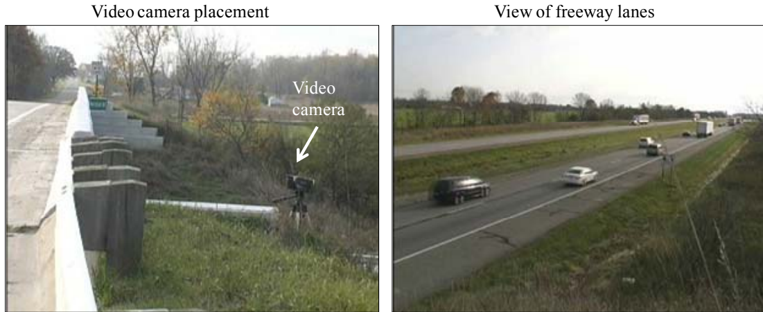
Figure 7. Typical video camera setup on sites east of Lansing
