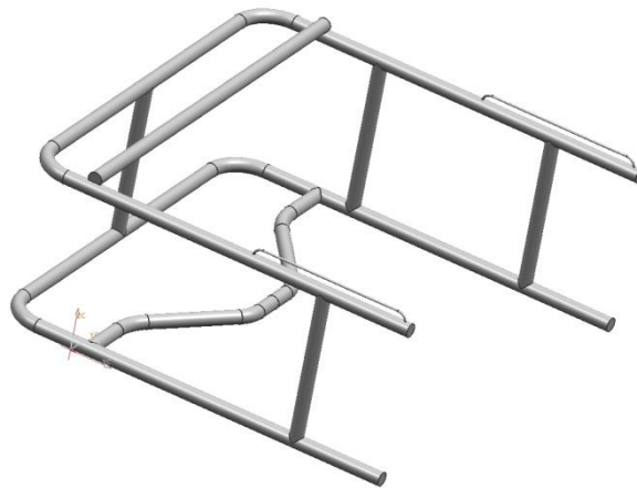
Figure 6.7: Proposed Frame for Pneumatic Scissor Lifting Mechanism
