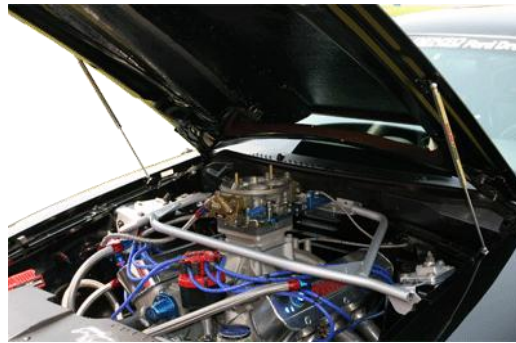
Figure 2.8: Gas springs used to assist lifting of a car hood [11]
