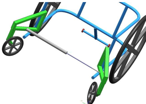
Figure 6.14: Isometric View of Extended Automatic Caster Mechanism
