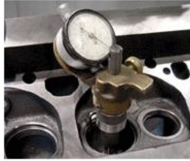
Figure 3.a: Left, probe indicator has a spring loaded probe with a displacement that is linear to the dial needle rotation. Right, the indicator with its mount on the engine block.
