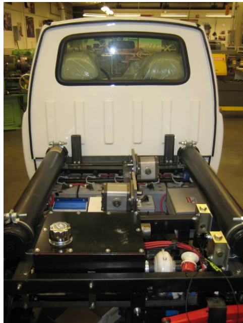
Figure E-2: Rear View of Installed Truck Components with Removed Truck Bed
