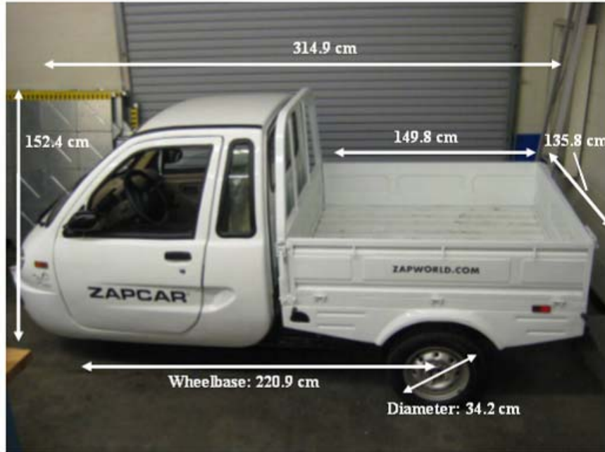
Figure 1: Xebra Electric Vehicle and Dimensions
