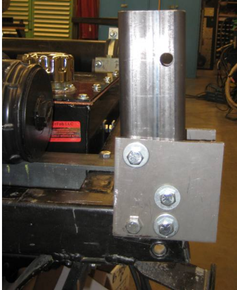
Figure E-3: Hinge Redesign with Truck Bed Removed
