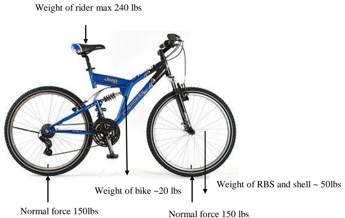
Figure 7: Free body diagram summarizing the various forces on the bike
