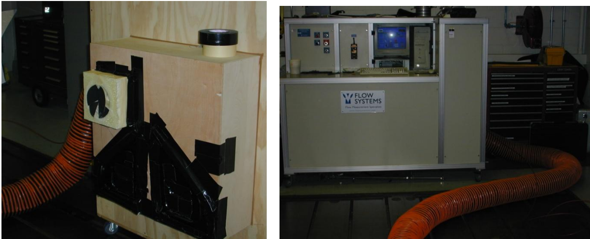
Figure 38: Sealed box with foam prototype attached (left), Flow Systems flow meter (right)
