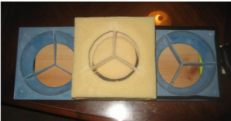
Figure 37: Final Prototype: Disassembled plastic prototype in blue with assembled foam prototype in yellow
