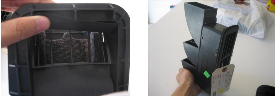
Figure 7: Sound deadening foam in Toyota Rav4 air extractor (left). Sound shield on Toyota Tundra air extractor (right)
