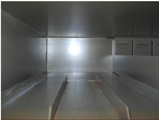
Figure 5: Simple Metal Tracks Used by Fisher Scientific to Restrain Movement of Drawers
