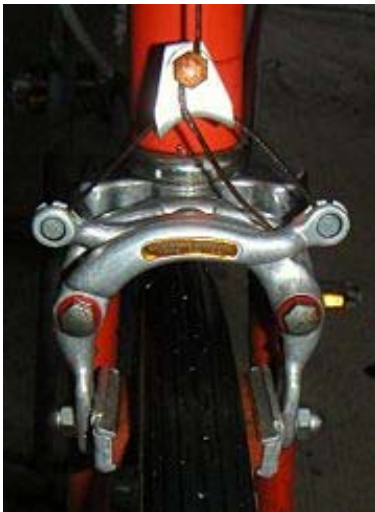
Figure 3. Center-Pull Cable on a Bicycle [9]
