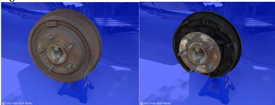
Figure 5: Drum Brake with and without Drum [10]
