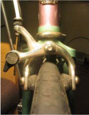
Figure 2: Side-Pull Cable on a Bicycle [9]
