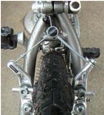
Figure 4: Cantilever-Pull Cable on a Bicycle [9]
