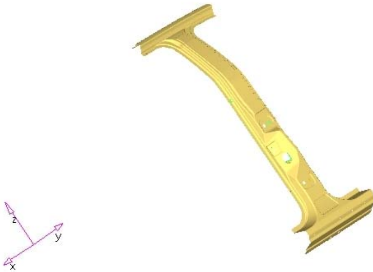
Figure 1: CAD model of Ford F-150 B-pillar.
