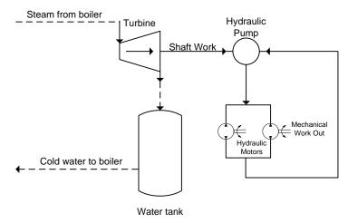
Running a hydraulic motor would be a similar process to generating electricity. However, because there is less power required for hydraulic motors, not as much energy would need to be extracted from the stacks. However, the hydraulic pump could be used in conjunction with electricity generation. The hydraulic pump would run the motors used to turn the furnaces and dryers.
