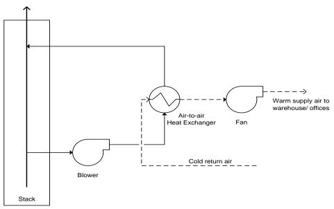
Heat for the offices and warehouse could be provided through a simple air-to-air heat exchanger. The flue gas passes through a cross-flow heat exchanger. The flow rate would be controlled to reach the temperature needed to heat the buildings. Blowers would be needed to overcome the pressure losses introduced by the system.
