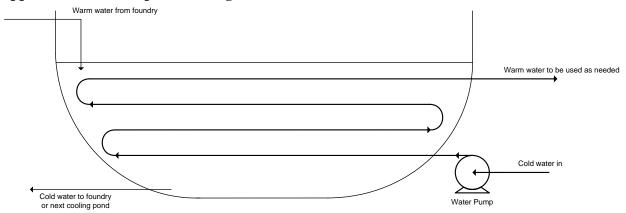
Appendix E.6: Concept 6: Heat Exchanger in Stack
