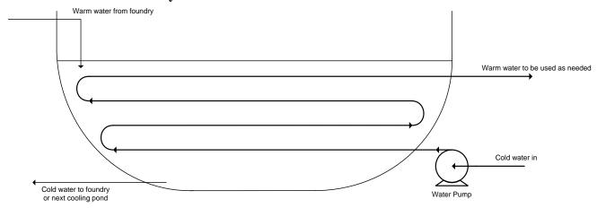
Hot water for use in the facility could be produced from the water in the cooling ponds. To accomplish this, water lines would be run through the cooling ponds with a pump. The hot water would be routed to the existing water heaters, where it would be stored and available to be used as needed. The cold water in the pond would be sent to the next cooling pond or to the foundry, depending on its temperature.
