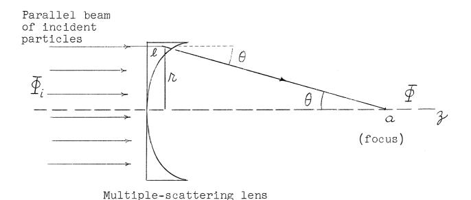
The geometry of a parabolic multiple-scattering lens.
