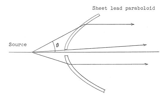
A paraboloidal lens of constant thickness for focusing particles diverging from a point source.
