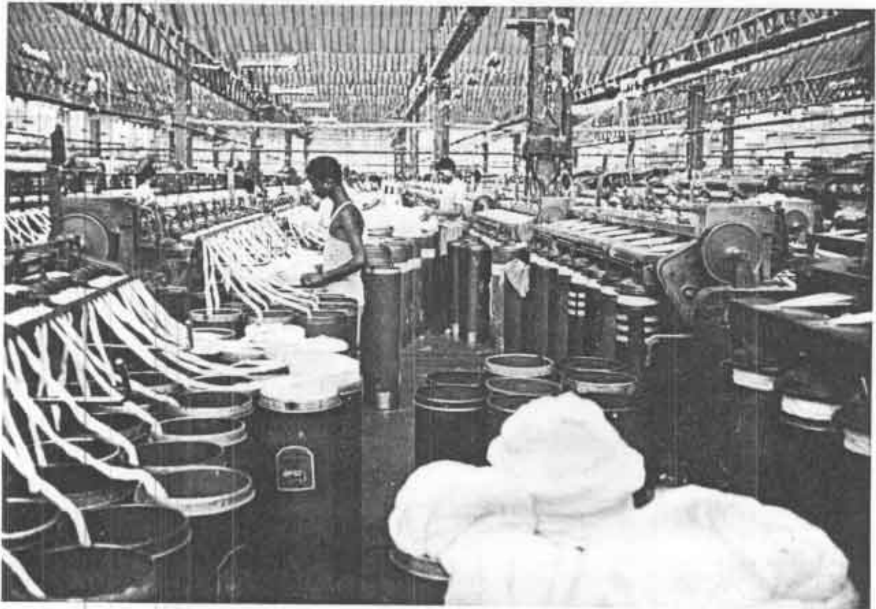
Figure 252. A view of the carding machines in the Keshoram Cotton Mills, Ltd., one of the largest textile mills in West Bengal. (Courtesy of United Nations.)
