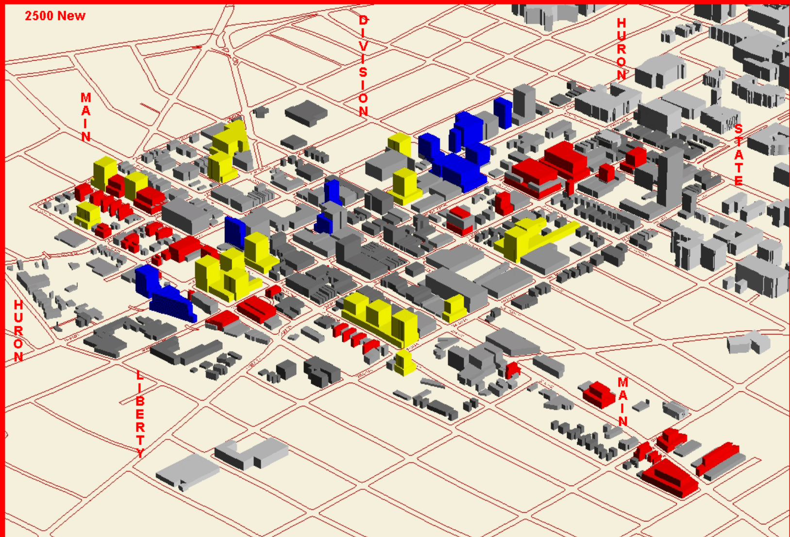
Figure 6.7a. Downtown Ann Arbor buildings extruded from footprints digitized from aerial. Gray buildings are existing buildings. Yellow buildings are built on empty lots or on surface parking lots. Blue buildings are built along Huron Street (possibly as replacements for, or on top of, existing buildings). Red buildings are built with upper story setbacks on a subset of streets identified by the Taskforce. The number of new buildings is sufficient to support 1000 new residential units. All non-gray buildings are built on prime parcels. Figure 6.7b: link to virtual reality model from which Figure 6.7a was taken.
