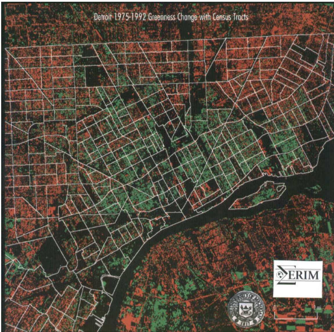
Figure 1. Landsat change image of Detroit showing changes in urban greenness from 1975 to 1992. Imagery and analysis are joint ventures between Environmental Research Institute of Michigan (ERIM) and The University of Michigan, College of Architecture and Urban Planning. Green areas show tracts with greenness increase; red areas with greenness decrease; black areas, no change. Change data derived from TM 1992 and MSS 1975 images of vegetation reflectance.
