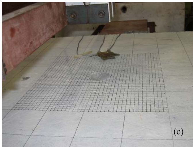
Fig 5.31 – Damage on the impact face of (a) R/C panel after 3 rd impact, (b) R/FRC panel after 7 th impact, and (c) R/ECC panel after 10 th impact (After [36])
