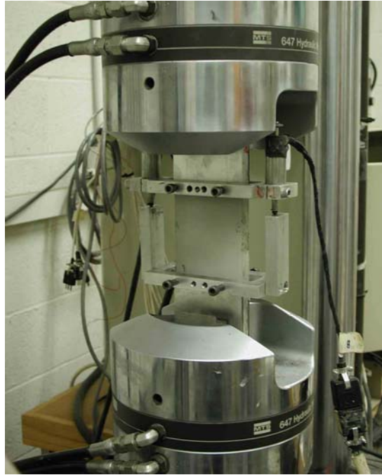
Fig 4.2 – Setup of the uniaxial tensile test
