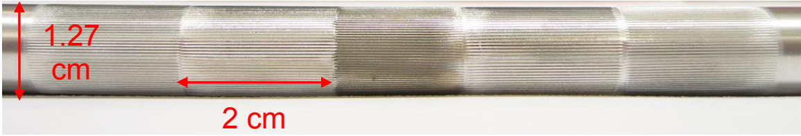
Figure 5.1 Ablated region of ALF-4b cathode showing “stacked” ablation rings to give 38 cm 2 of total emission area.
