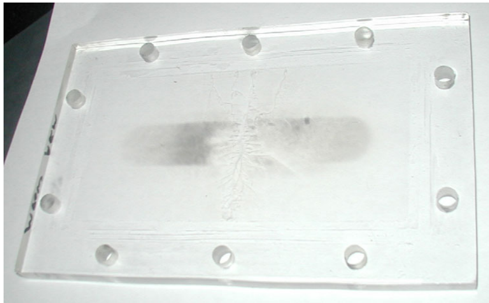
Figure 4.6 Output waveguide window exhibiting breakdown on the vacuum-side of the window. The dark outline shows the size and shape of the magnetron coupling slots.
