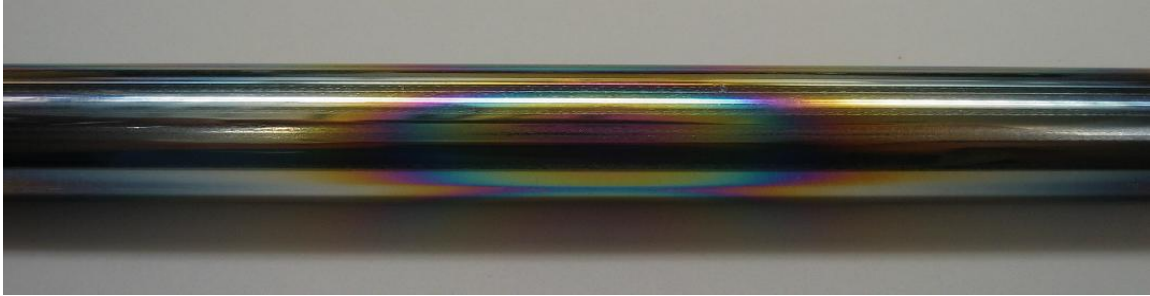
Figure 3.20 Photograph of the patterned region of the dielectric coated cathode. The cathode diameter is 1.77 cm.
