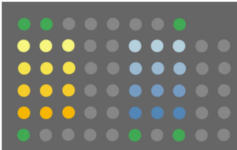
Figure 4.10 Schematic of a constellation design where arrays of the DNA oligonucleotides, RCm and NCm (yellow and blue circles), are printed in rows of increasing concentration (0.5 \mu\text{g}/\mu\text{l} , 1.5 \mu\text{g}/\mu\text{l} , 5.0 \mu\text{g}/\mu\text{l} , and 15 \mu\text{g}/\mu\text{l} ). Green circles indicate calibration spots composed of a 0.5 \mu\text{M} mixture of RCm and NCm. Grey circles indicate buffer spots.
