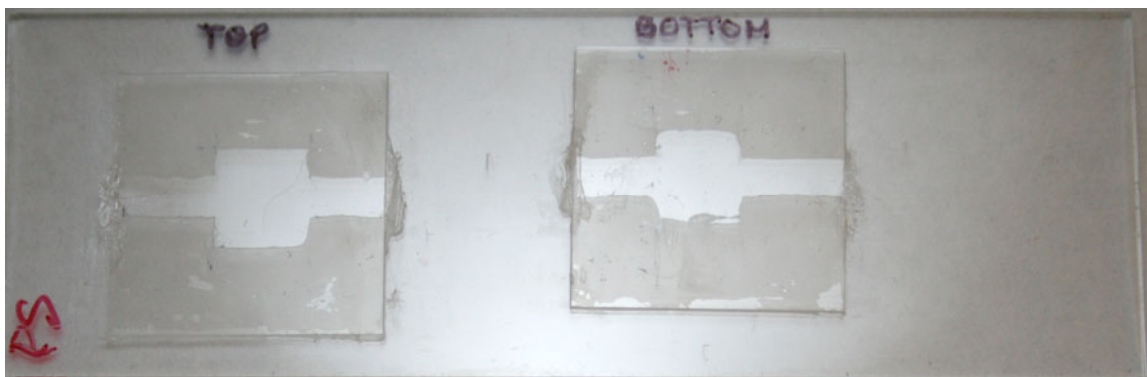
Figure 4.11 Microarray flow cells. Two microarray constellations are printed on each glass slide. The constellations are surrounded by a parafilm channel, atop which the coverslip is placed. The parafilm is melted using a soldering iron, adhering the coverslip to the slide and creating a flow channel for measurements in a fluid environment. Once fluid is introduced into the channel, the inlet and outlet are sealed using vacuum grease.
