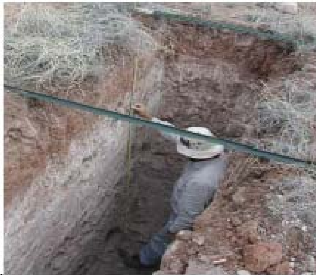
Fig. 1.1: An example of layered soil profile in WGEW, showing the rough interfaces and visible moisture variations within each layer
