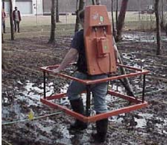
Fig. 1.2: Detection and localization of unexploded ordnance (UXO) using ground penetrating radar (GPR)
