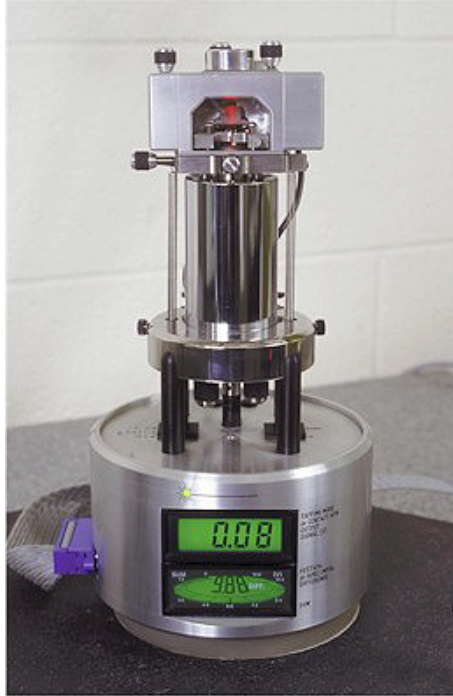
Figure 3.14: Digital Instruments Nanoscope III TM Multimode Scanning Probe Microscope, in combination with the Atomic Force probe.
