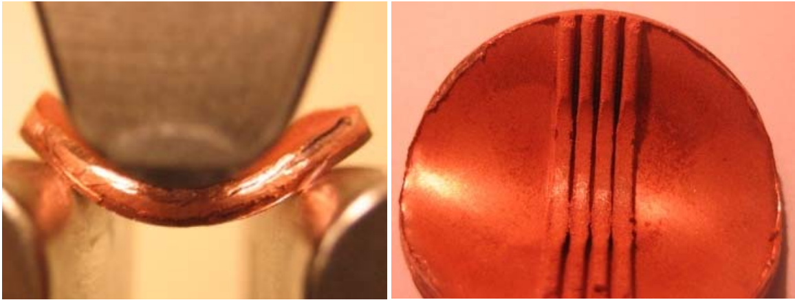
Figure 3-23 Three-point bending test
