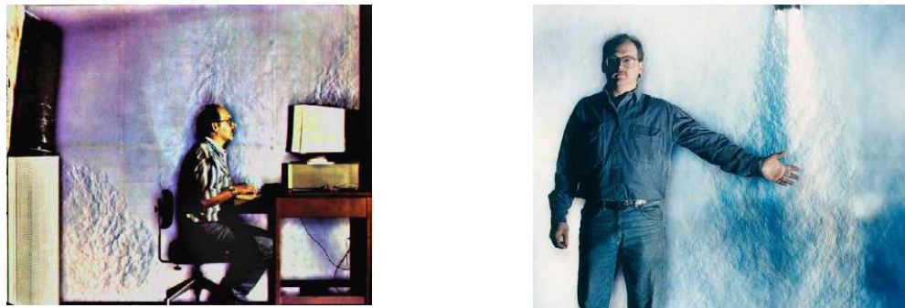
Figure 11 Airflow patterns captured by Schlieren and Shadowgraph techniques [29, 30]
