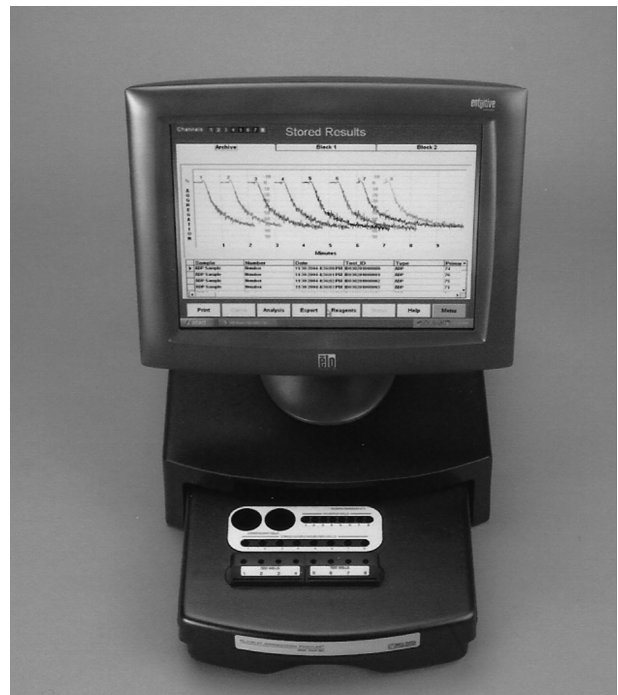
Figure 1: Turbidometric platelet aggregometer. It measures the decrease in light transmittance that results from platelet coaggregation in platelet-rich plasma, when samples are exposed to an agonist such as ADP. Reproduced with permission from Harrison P et al. 5
