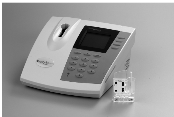
Figure 3: The VerifyNow platelet aggregometer. Reprinted with permission from Harrison P et al. 5
