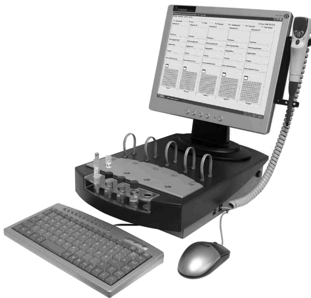
Figure 2: Impedance platelet aggregometer. It measures the increase in electrical impedance across two precious metal wires that results from platelet coaggregation in whole blood, when samples are exposed to an agonist such as ADP. Reproduced with permission from Harrison P et al. 5
