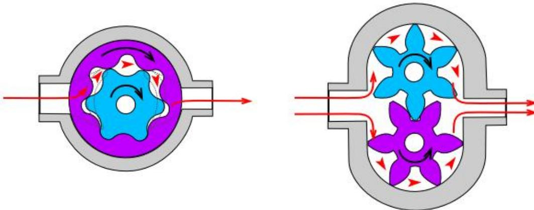
Figure 2: Gerotor Pump (left) and Spur Gear Pump (right) fluid flow schematics (Wikipedia, 2008).
