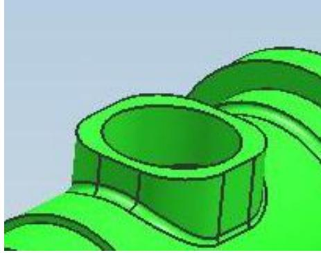
**Figure 29: Outlet Line Bung on Water Pump Adapter**
