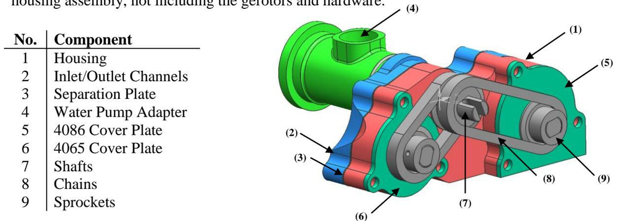
Figure 21: Housing Assembly and Components
