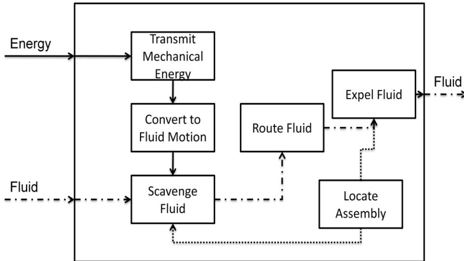
**Figure 7: Level II functional decomposition illustrates the specific tasks that need to be accomplished.**
