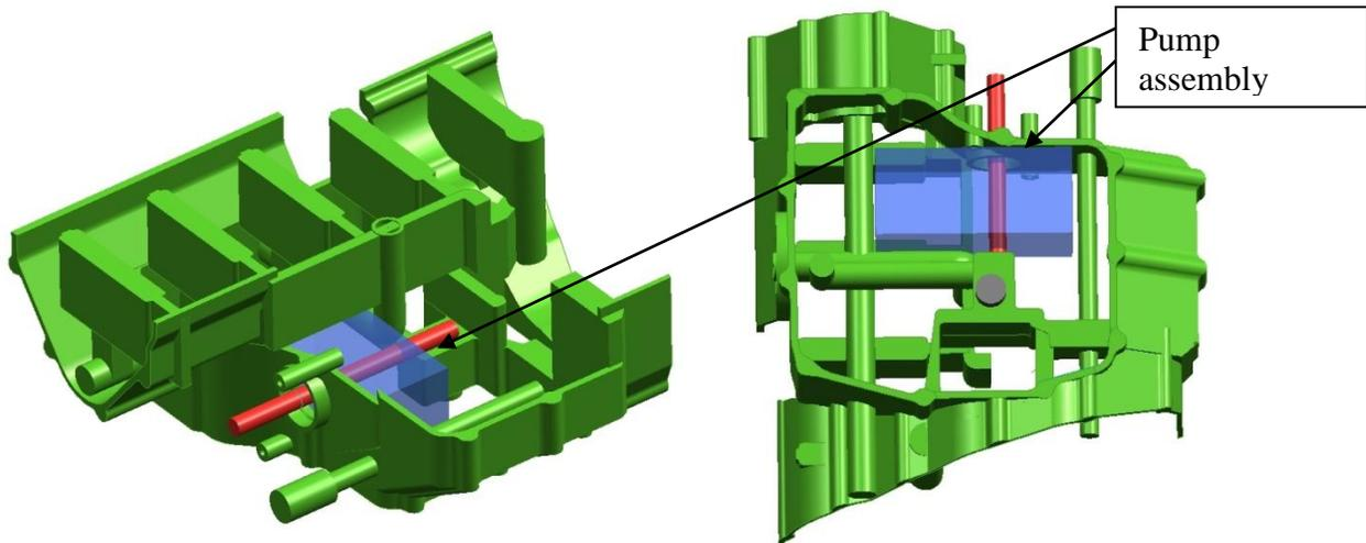
**Figure 4: Isometric (left) and bottom (right) views of the required pump assembly location.**
