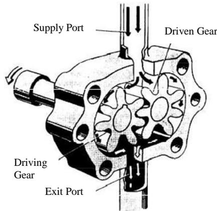
**Figure 10: Spur gear style pumps use two meshed gears, one driveshaft and one driven shaft to pump fluid through housing. [2]**
