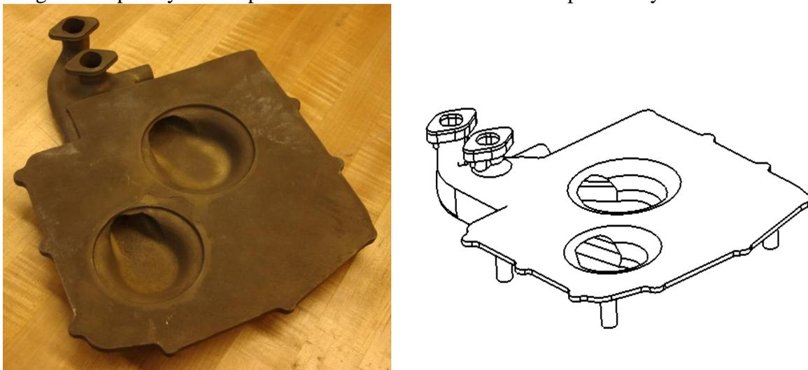
Figure 1: Picture (left) and schematic (right) of the 2007 oil pan showing oil collector pockets
