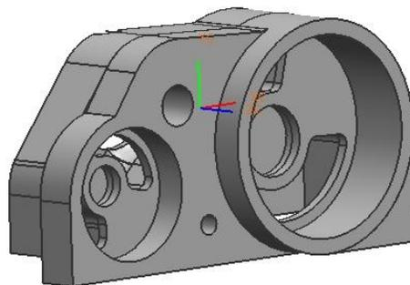
**Figure 20: Design which makes use of different sized gerotors to match stream of oil in crankcase.**
