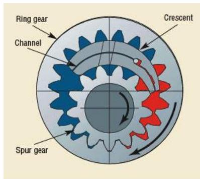
**Figure 11: Crescent style pumps use internal gears and one driveshaft, similar to the gerotor. [3]**
