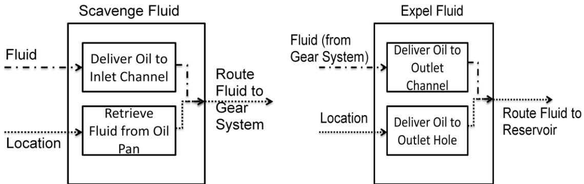
**Figure 8: Level III functional decomposition demonstrates further classification of scavenge requirements.**
