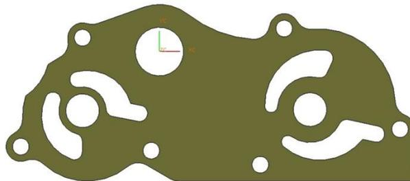
**Figure 24: Separation plate has Nichols Portland defined porting geometries**
