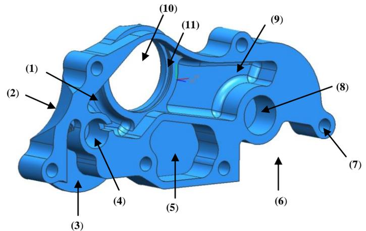
**Figure 23: Inlet outlet channel features**
