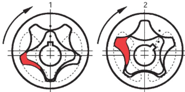
**Figure 9: Gerotor style pump uses two rotors and one driveshaft to continuously pump fluid in and out of the chambers. [1]**
