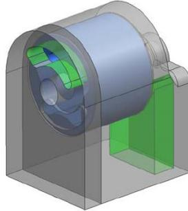
**Figure 13: Concept utilizes a direct drive method exhibits a single stage and long inlet channel.**
