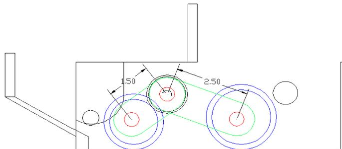
**Figure 14: Sketch of shaft and gerotor configuration was used to determine the optimal power transmission method.**
