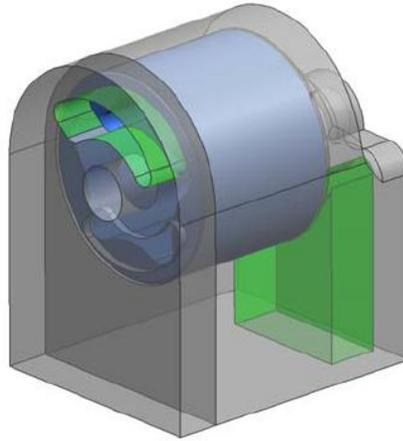
**Figure 17: First iteration of scavenge pump satisfies capacity requirements, but falls short of other requirements.**
