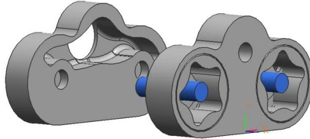
**Figure 19: Exploded view of the first two-stage iteration highlights two side-by-side gerotors and an elegant outlet channel.**
