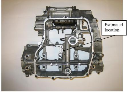
Figure 3: Estimated location of maximum oil scavenging capacity
