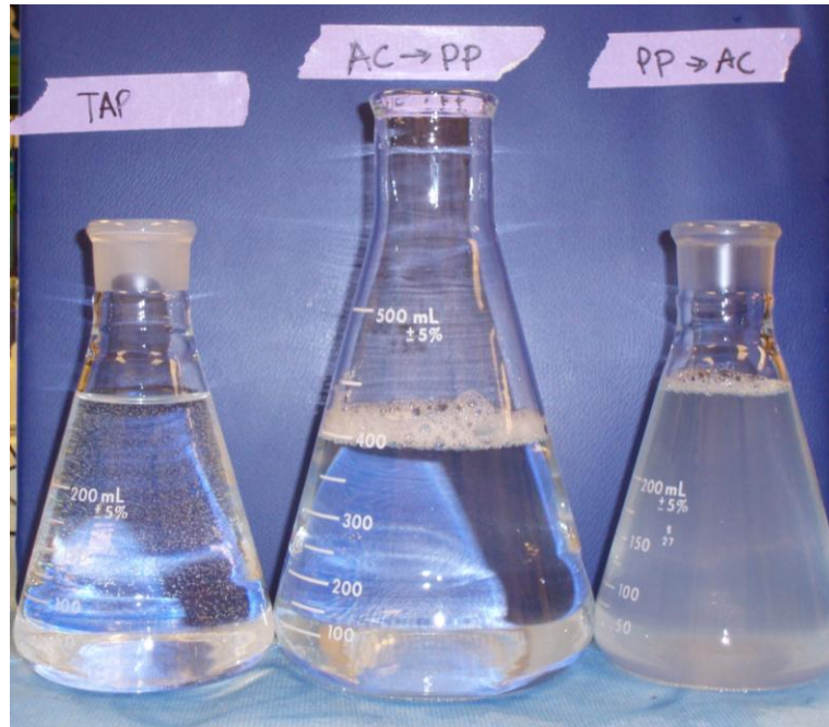
Figure B.3. Shows Trials 4 (AC→PP) and 5 (PP→AC) compared with tap water. Trial 4 can clearly be seen as similar to tap water turbidity.
