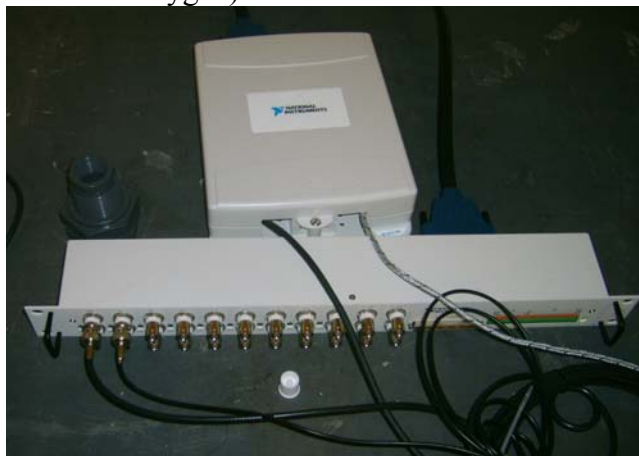
Figure 20: Terminal blocks of PCI-6225 data acquisition card with sensors connected
