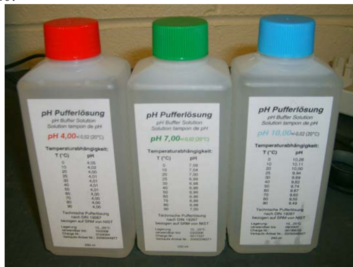
Figure 26: Reference pH solution with values of 4, 7 and 10.
