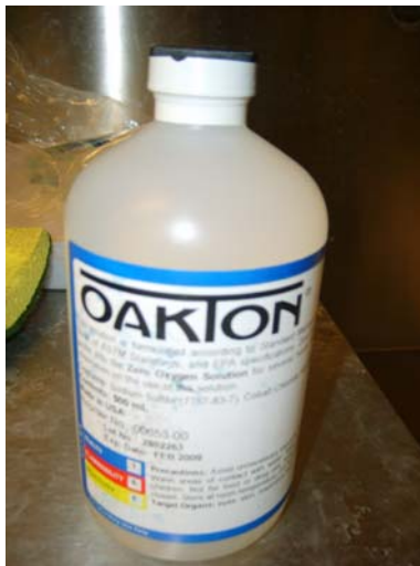
Figure 30: Zero dissolved oxygen solution.
