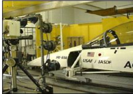
Figure 10: FOD Testing of F-15 Windshield
