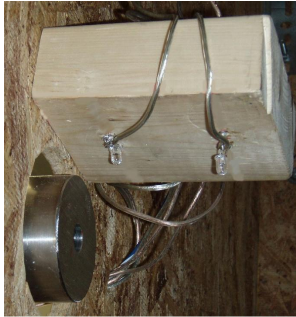
Figure 4: Setup of velocity measurement system
