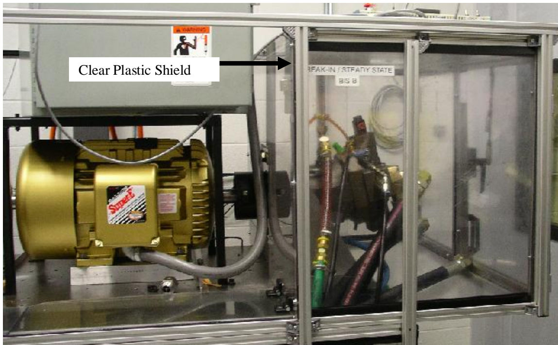
Figure 1: Current safety shielding used to confine hydraulic equipment
