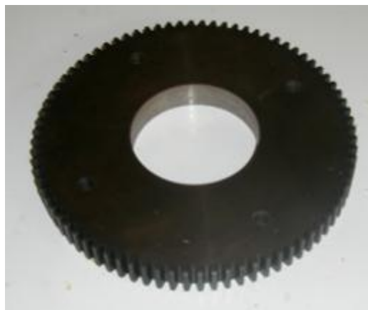
Figure 50: Main gear 1/4in hole locations
