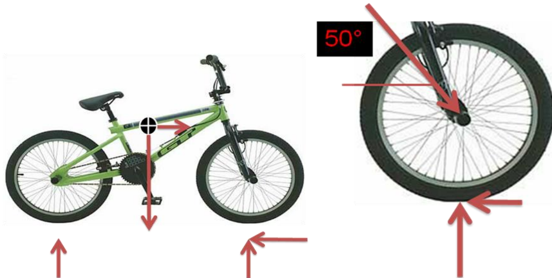
Figure 71: Free body diagram of the forces acting on the braking bicycle. A close-up of the front wheel is also included with the forces acting on it
