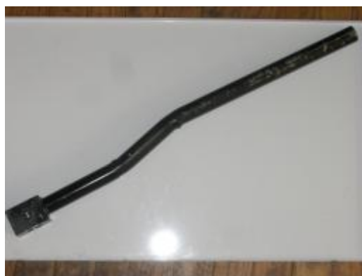
Figure 45: Side view of custom bent axle
