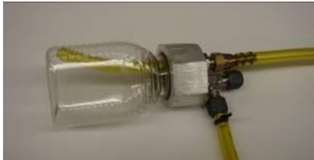
Figure 35: Low pressure accumulator with cap and fittings
