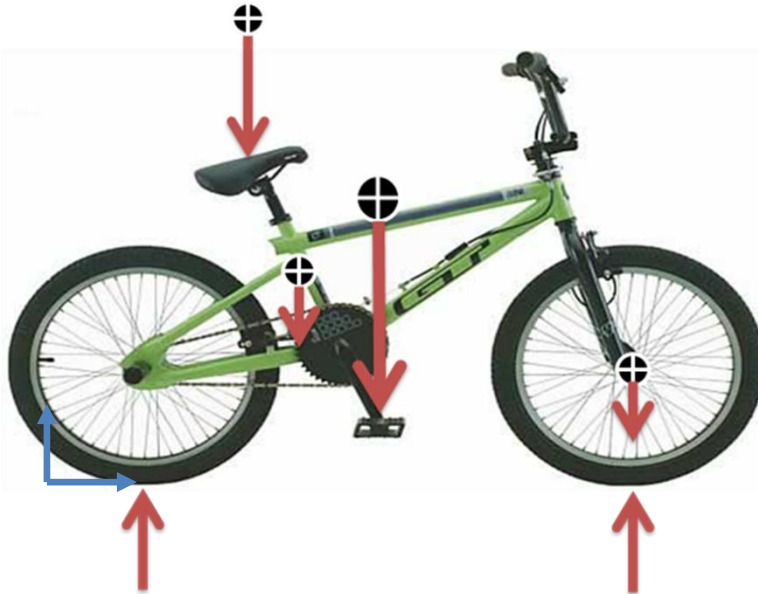
Figure 23: Static free body diagram of the 20" bike
