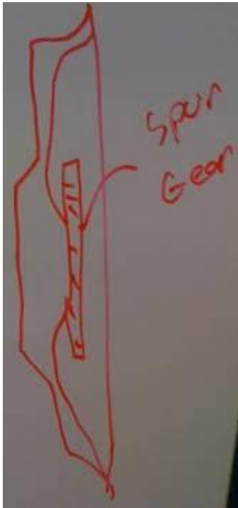
Figure 70: Hub design concept in which the spur gear is machined directly onto the side of the hub shell, to eliminate the extra spur gear purchase.
