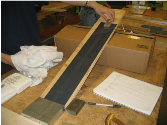
Figure 31. Inclined plane friction test
