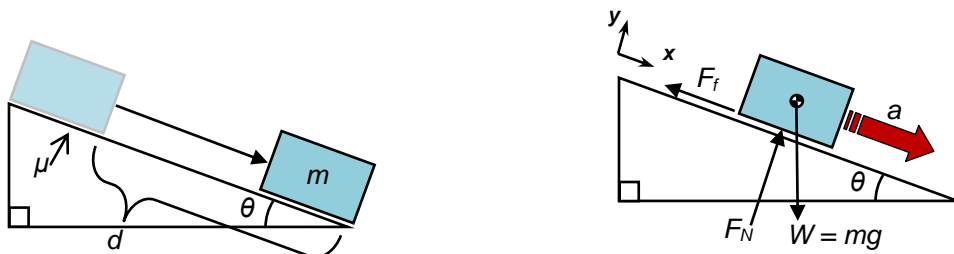
Figure 21. Inclined plane experiment to determine \mu for test surfaces with free body diagram (right)
