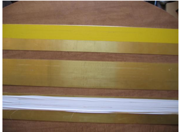
Figure 32. Friction surfaces: duct tape (top), packaging tape (middle), Teflon tape (bottom)
