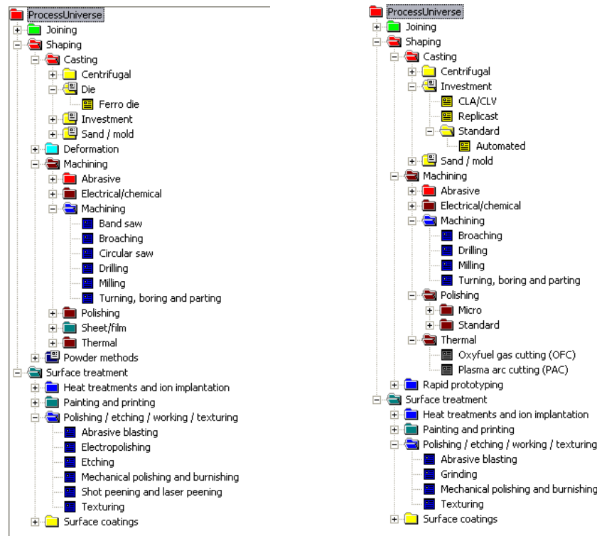
Figure 43. CES Manufacturing Process Selector recommendations for Cam (left) and Brake Shoe (right)
