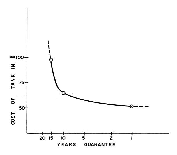
FIG. 3 - RELATIONSHIP BETWEEN COST OF HOT WATER TANK AND GUARANTEED LIFE.
