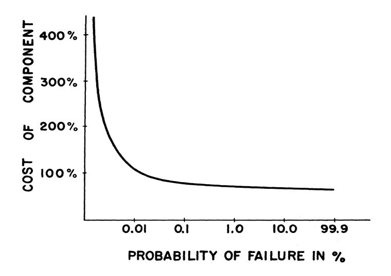
FIG.2 - RELATIONSHIP BETWEEN COST AND PROBABILITY OF FAILURE.
