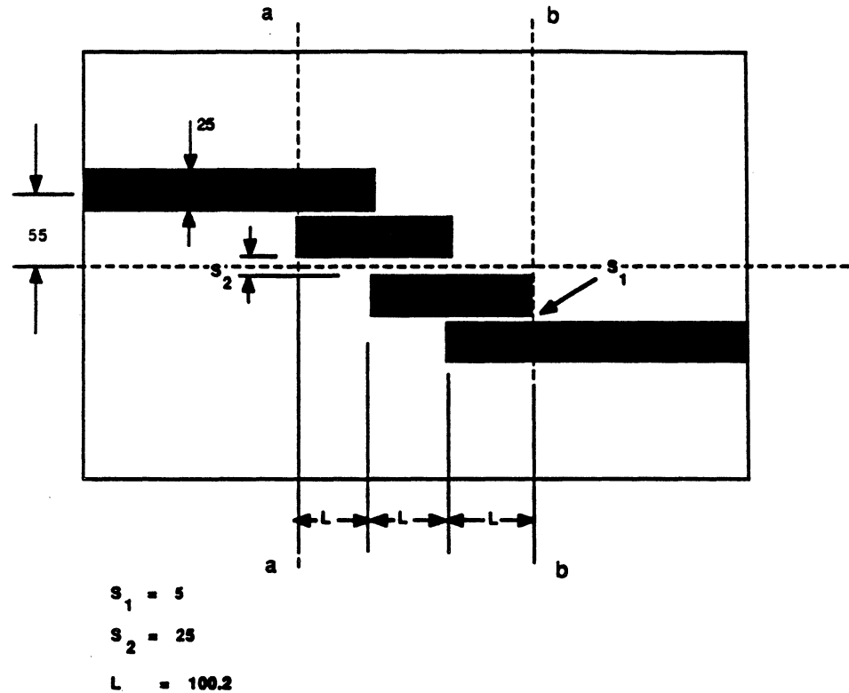
Figure 4.11: Sketch of two resonator coupled line filter. Note: all dimensions in mils, h = 25 , \epsilon_r = 9.7 . (Shielding dimensions: b = .4'' , c = .25'' ).
