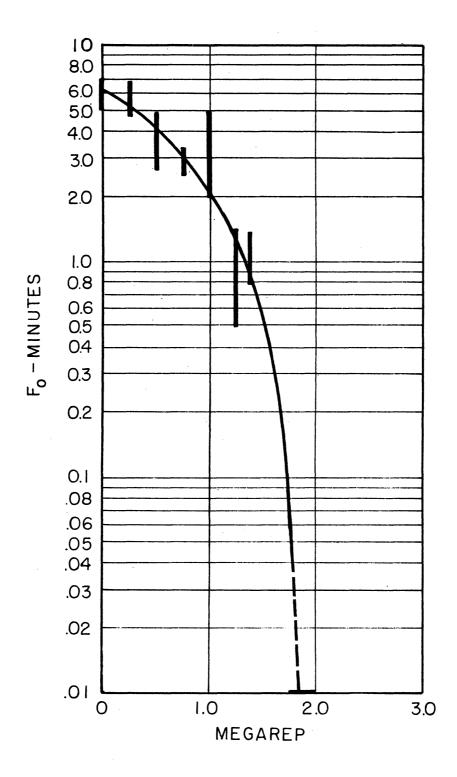
$F_O$  required to sterilize cooked ground beef packed in No. 1 picnic cans, inoculated with 300 PA-3679 spores per can, and irradiated with gamma rays from cobalt-60 before heat-processing at 230°F.
