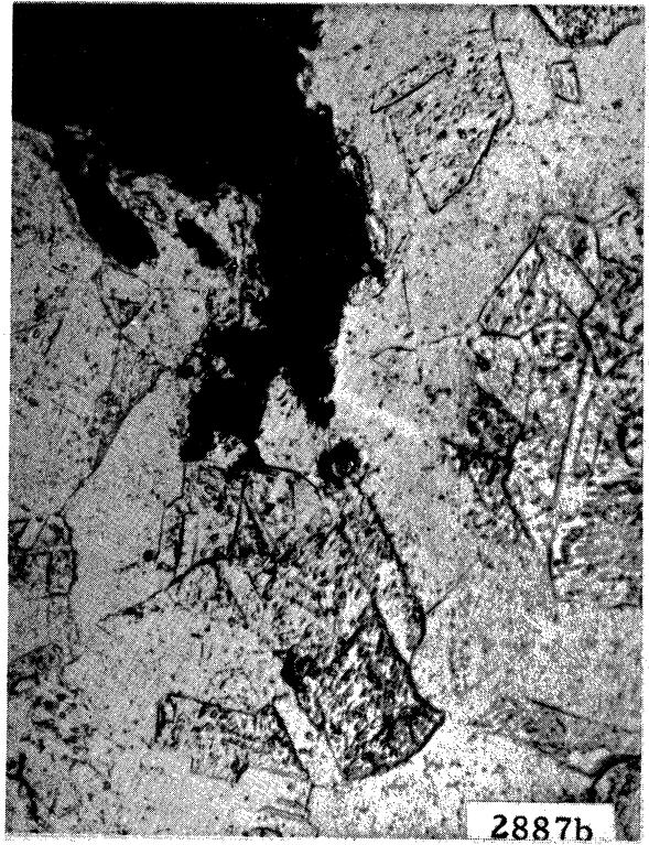
Figure 19. Photomicrographs of Cavitation Damage Area of Compression OFHC Copper Vibratory Specimens (400x)
