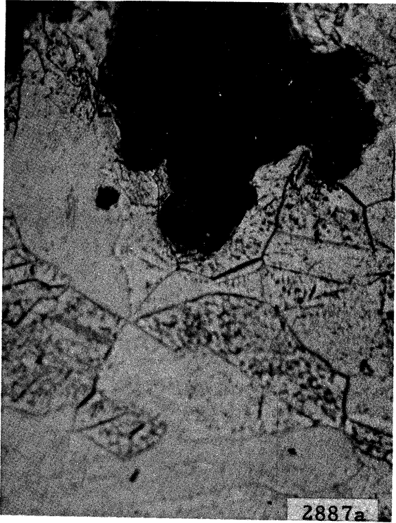
Figure 19. Photomicrographs of Cavitation Damage Area of Compression OFHC Copper Vibratory Specimens (400x)
