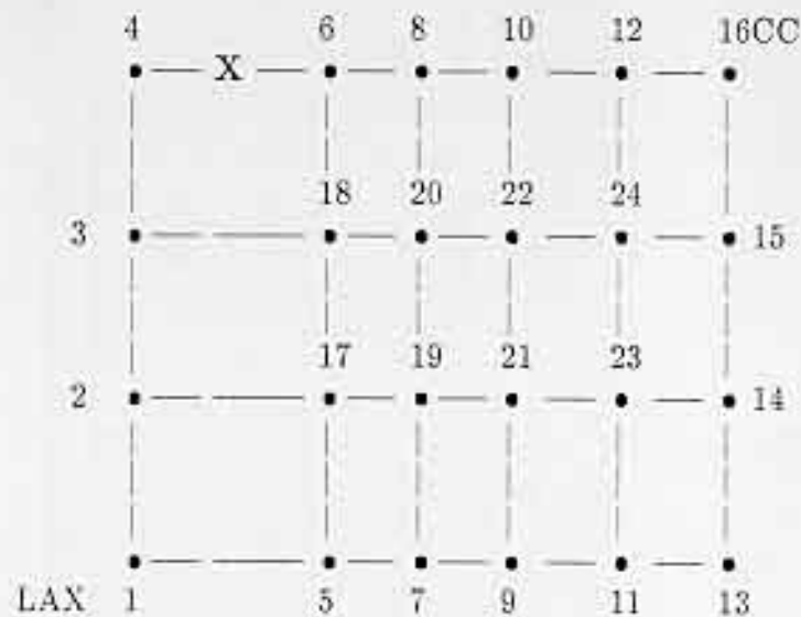
Figure 3. Same basic pattern as Figure 1, with surface routes added, and intersections of surface routes added as nodes in the graph. LAX denotes Los Angeles International Airport. CC denotes the Central City. Routes are along major expressways. The X indicates the rupture in the Santa Monica freeway caused by the January 17, 1994 earthquake. Consider that all lines, whether dashed or solid, represent continuous graphical linkage between adjacent nodes. The only break in the freeway is at the X.
