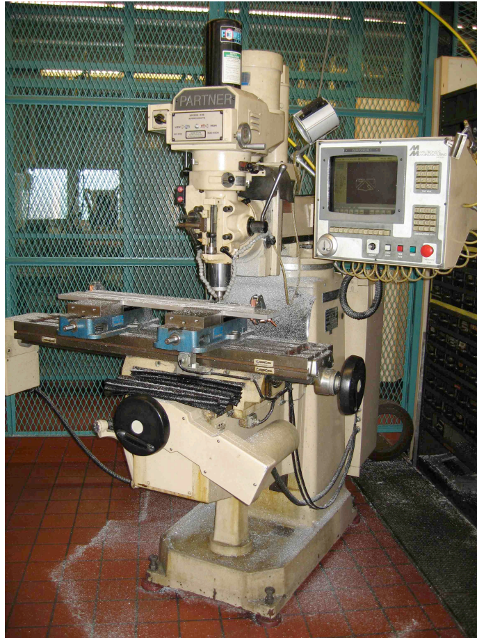
Figure 5.6: Machining of compliant mechanism structure on 3-axis CNC mill
