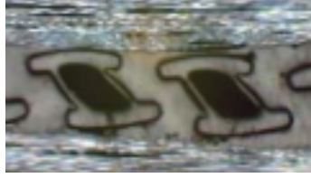
Figure 1.5: Cross-section of machine augmented composite, from Hawkins et al. [37]
