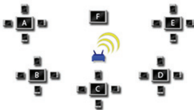
Figure 3. A schematic depicting the use of MUSHI-LIFE in a classroom of 20 students. The students each have a handheld computer and are divided into five groups of four. These five groups each surround a tablet or desktop PC running MUSHI-LIFE, labeled A-E. The remaining tablet or desktop PC, F, is reserved for the instructor's use. A wireless access point allows the devices and PCs to communicate with one another wirelessly.
