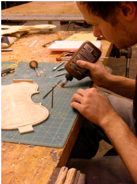
fig. 21 Applying glue to a strip of maple, that will be placed between two pieces of ebony.
