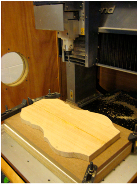
fig. 41 A spruce blank set up in the milling machine. After the top side of the piece is cut, it will be flipped over for the other side to be cut.
