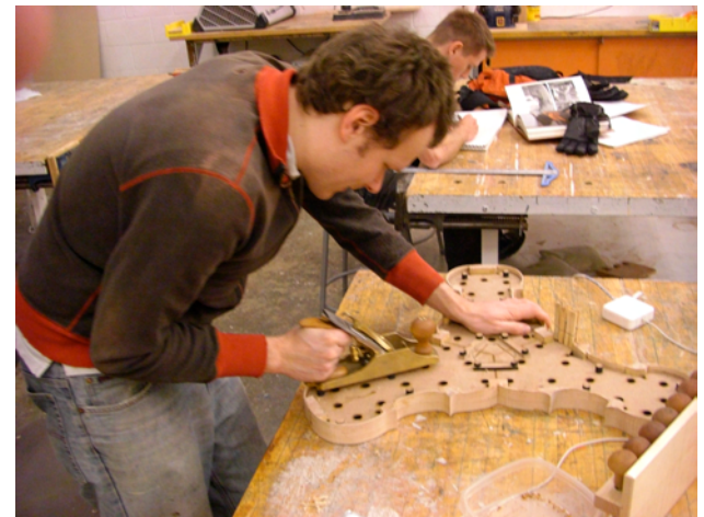
fig. 55 Cleaning the edges of the ribs to be parallel with the corner blocks. It was good to have a very sharp plane, because certain areas had me cutting against the grain.
