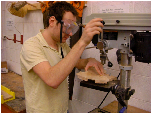
fig. 27 The ends of the “F” holes are drilled out on a drill press.
