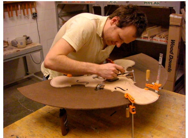
fig. 45 The three top plate are glued and clamped together.
