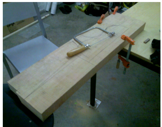
fig. 19 The rough cut Sitka Spruce that will eventually become the top plates and the internal blocks. If you look closely you can see several halved violin profiles, and the coping saw used to cut them out.
