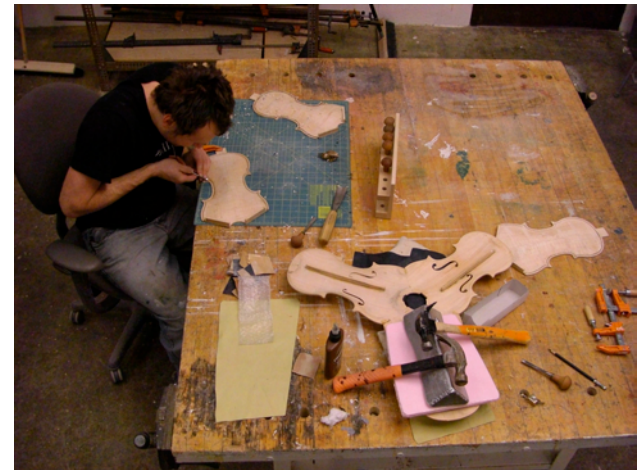
fig. 24 Carefully cleaning access material out of the corners of the plate.
