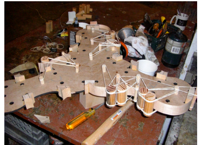
fig. 53 Several ribs glued and clamped. I could not glue all of them at once because there was extra material that had to be removed from each piece before the next could be put in place.
