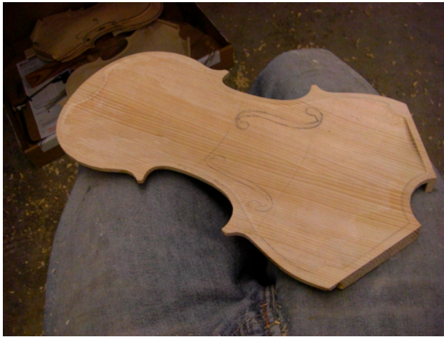
fig. 26 The plate is reasonably tuned and the “F” holes are drawn on for reference. The tabs at the back of the plate are left on to provide a clamping area.
