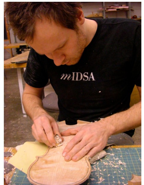
fig. 25 I am removing all traces of the glue tabs, and shaping the surface into its final contours. The curly maple grain alternates very violently. Which makes it very difficult to use any kind of cutting tool accurately.
