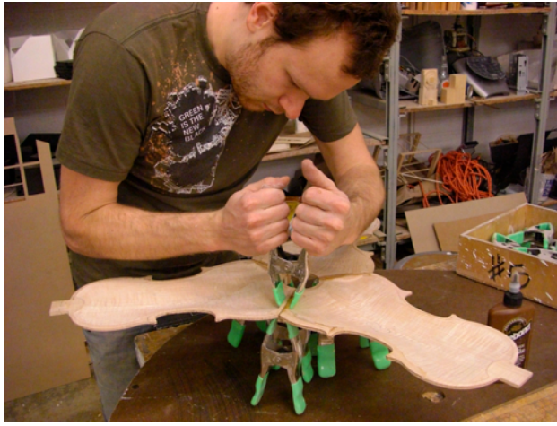
fig. 47 Clamping the bottom plates. The second time around I improved my clamping strategy.
