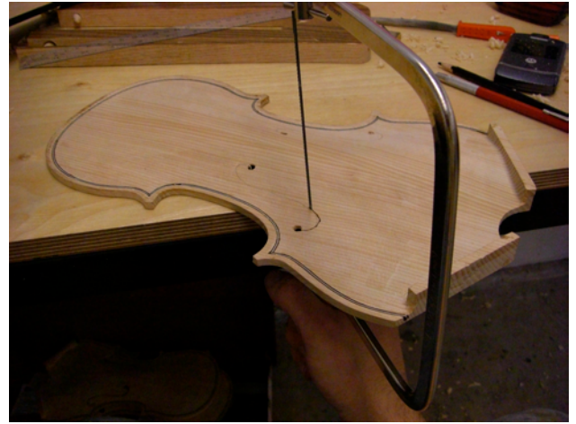
fig. 28 The “F” holes are shaped by sawing out a connection between the two drilled holes.
