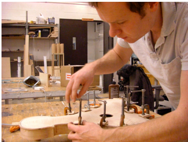
fig. 57 Glueing the bottom plate to the ribs. It took a lot of clamps to distribute even pressure along the entire edge. Luckily hide glue has a longer working time than regular wood glues, which afforded me the time to make things perfect.
