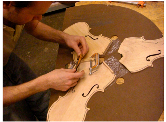
fig. 44 Clamping the top plates together. Notice that the piece on right does not have clamping tabs. This is because that section was made entirely by hand while the other two were digitally assisted.
