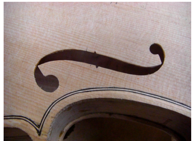
fig. 30 The final shape of the “F” hole, including notches.
