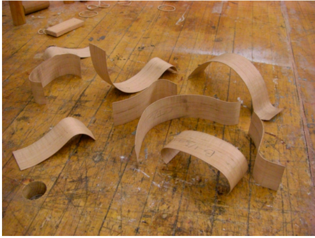
fig. 51 A group of bent ribs before they are glued on the jig.
