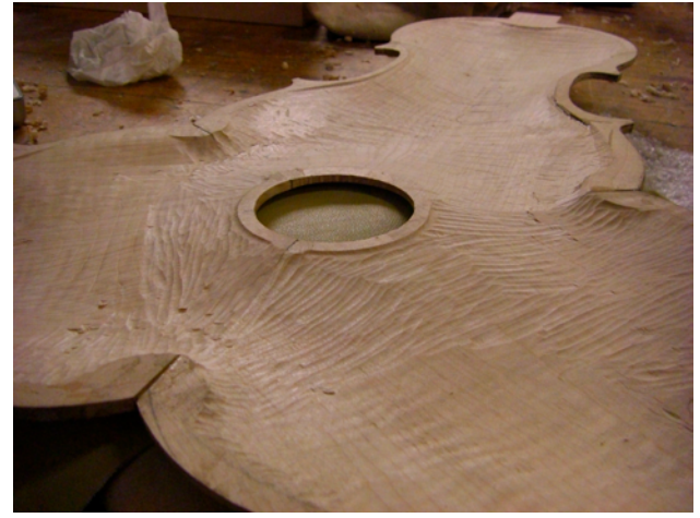
fig. 48 The internal tabs removed, with evidence from the palm gauges is still present. The section will be seamlessly blended together using finger planes and scrapers.
