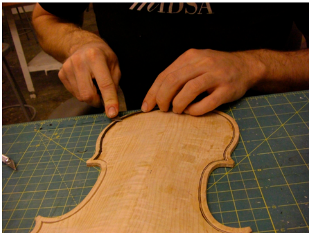
fig. 22 Pressing the purfling into place. If it does not fit all the way down, then there is a chance that it will get torn later in the carving process.
