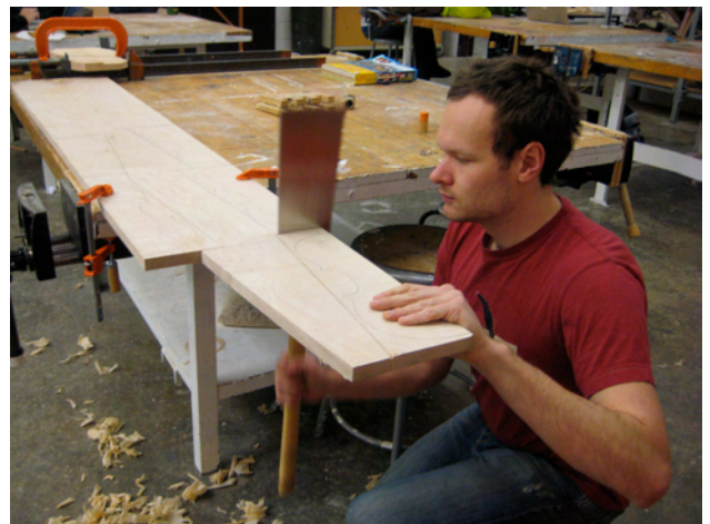
fig. 21 Freeing a halved violin plate from the maple board.
