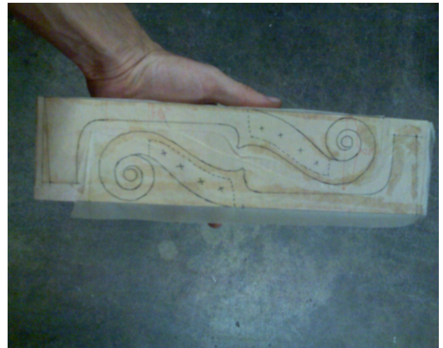
fig. 17 Two scroll patterns adhered to a block of curly maple wood. After sawing the necks free from the block, the scrolls are carefully carved by hand.
