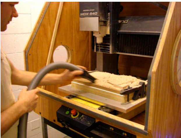
fig. 43 The volume of saw dust from the mill is at least 5 times the volume of the original piece. A strong shop vacuum is needed to free the plate from its former self.
