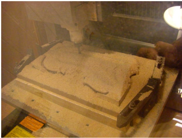
fig. 42 The belly of a top plate being worked on by the mill.
