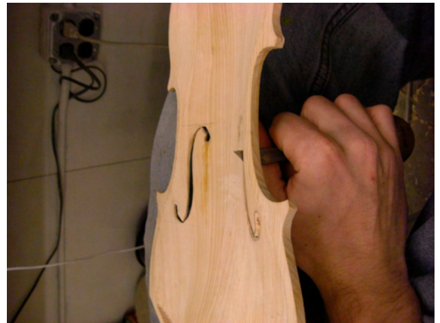
fig. 29 The Holes are expanded to their final shape and size with a knife or a skew chisel.
