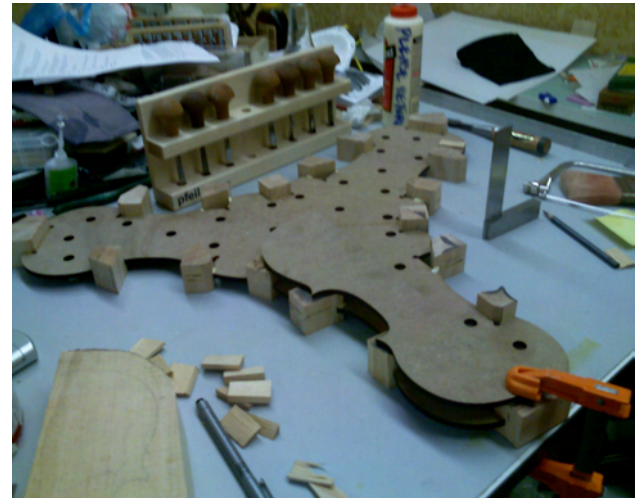
fig. 49 The physical jig with blocks glued into place. There is a stencil on top of the blocks nearest to the camera. After tracing around the stencil, all the material that does not follow the curve will be removed.
