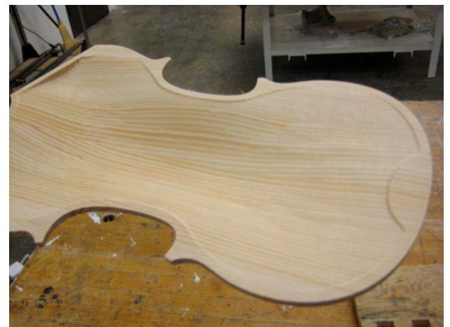
fig. 40 The backside of the top plate. The thickness of the entire piece is 5 mm, it will be worked by hand down 2.8 mm in some areas. The plate is tuned during this process, revealing its pitch, tone and resonance. There is an area around the edge that is saved as a glueing surface for the blocks and ribs.
