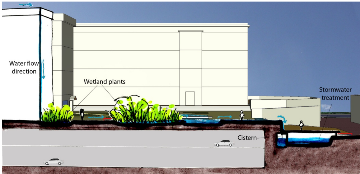
Figure 5.16 Elevation of the stormwater treatment
