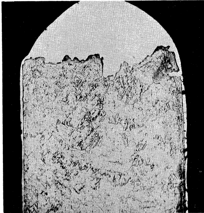
Fig. 33. Copper specimen fractured at 650°F in 100% bismuth environment. 50X
