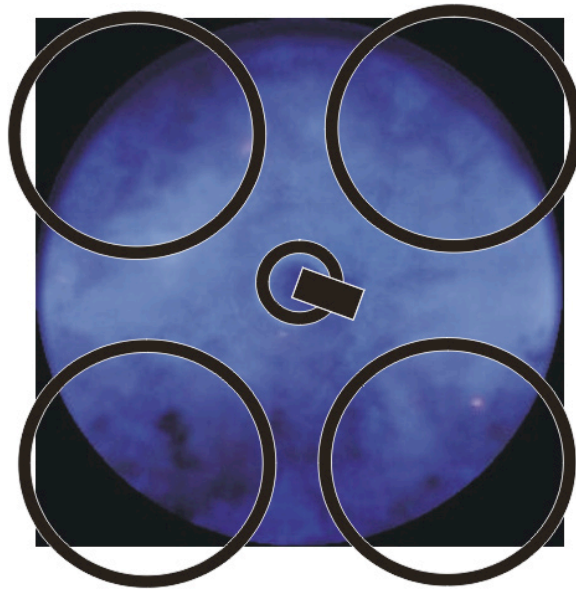
Figure 2.5: Orientation of the imaged frames with respect to the cylinder geometry. Intake valves are on the bottom, and exhaust valves on the top. The spark plug is shown at the center.
