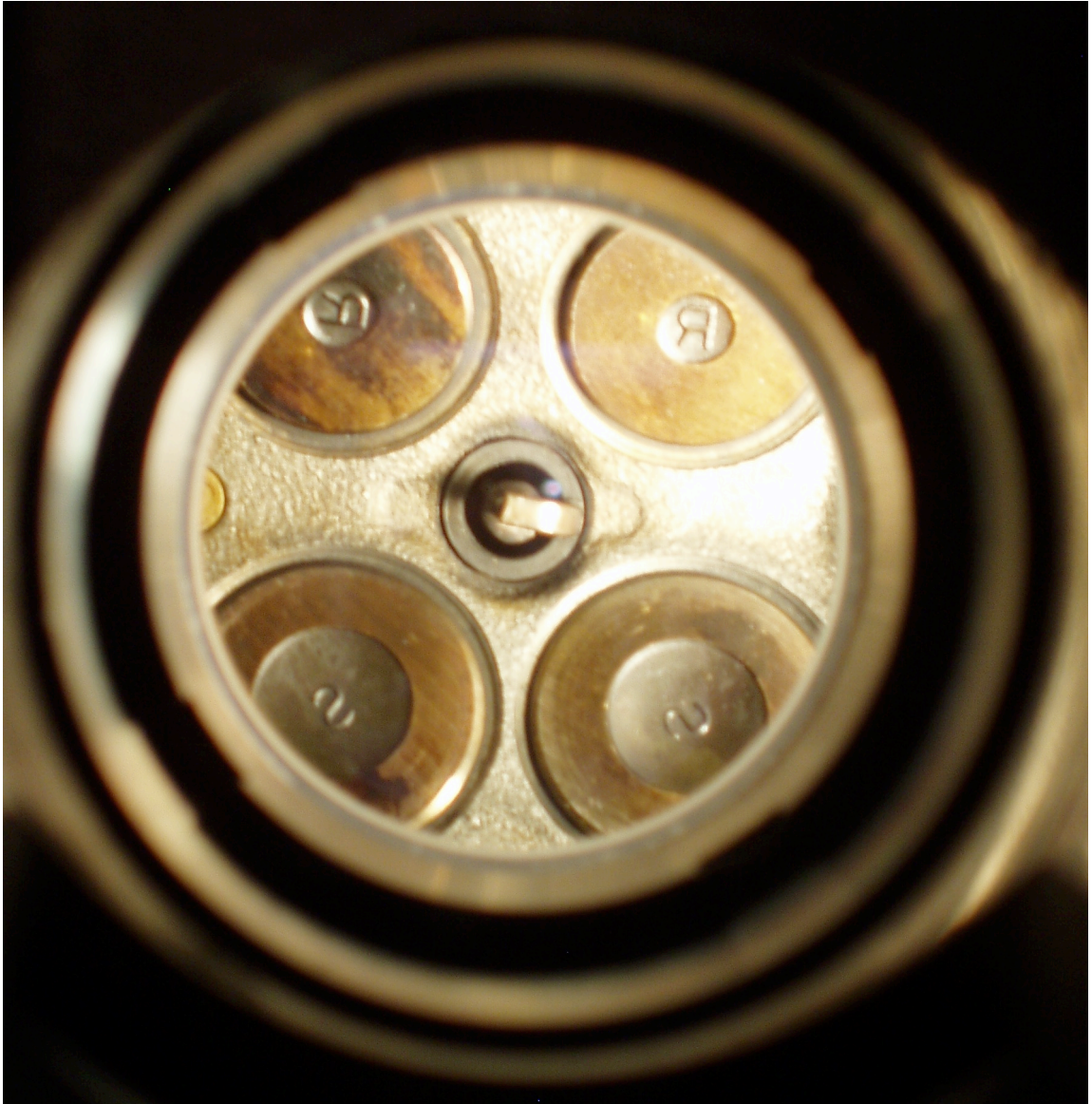
Figure 2.3: View of the intake valves (top), exhaust valves (bottom), and centrally mounted spark plug, as viewed through the mirror and piston window.
