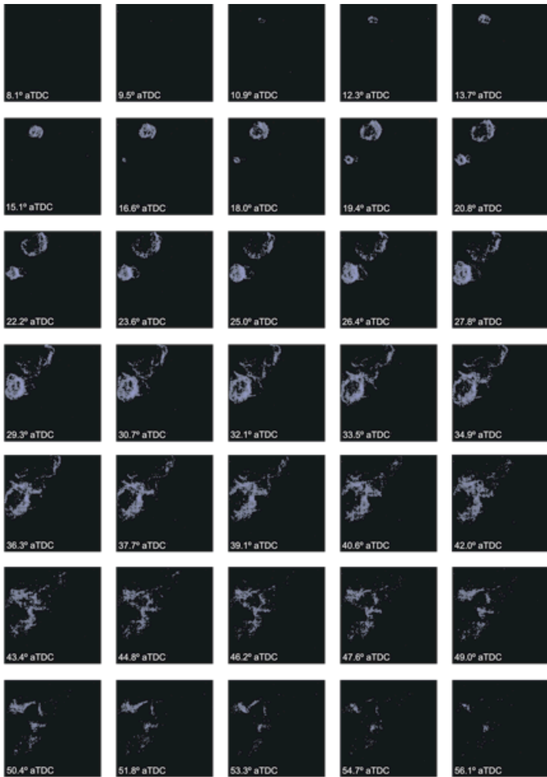
Figure 4.6: Typical piston view image sequence for weak HCCI combustion. T_{int} = 271\text{ }^{\circ}\text{C} , \phi = 0.62 , with indolene fuel.
