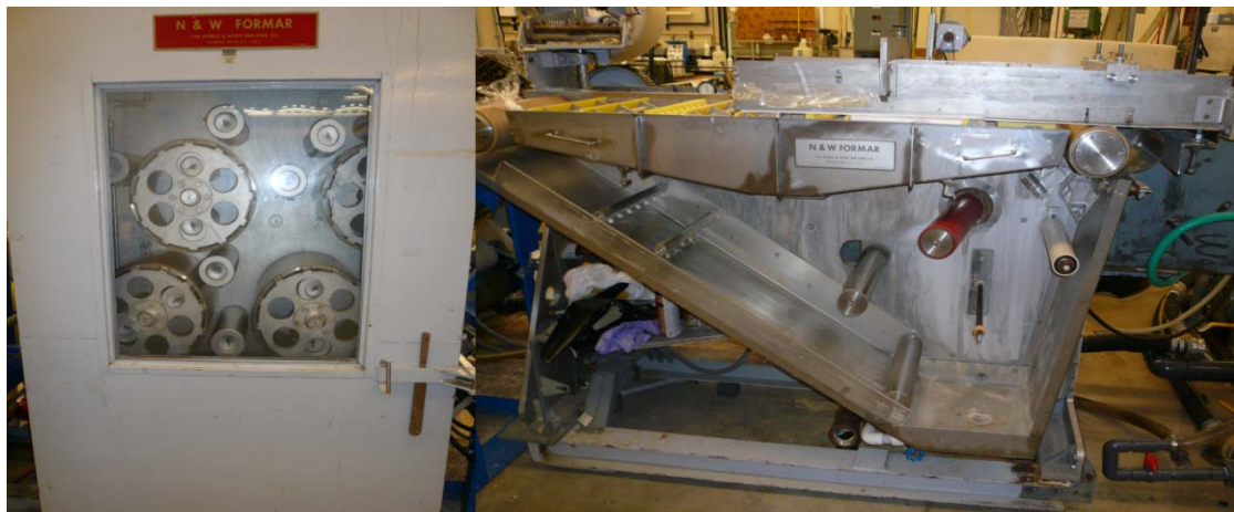
Figure 5.8 Dryer (left) and former (right), both without belts at the University of Washington.
