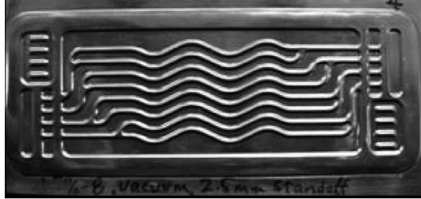
Figure 1.1: A 316L stainless steel sample formed electromagnetically using a uniform pressure actuator (courtesy of Dr. J. R. Bradley, General Motors Research and Development).
