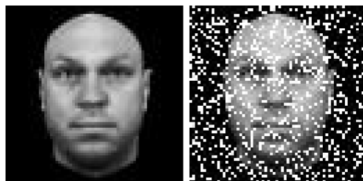
Figure 4.1: The original face image (left panel) and the corresponding image corrupted by impulse noises (right panel).
