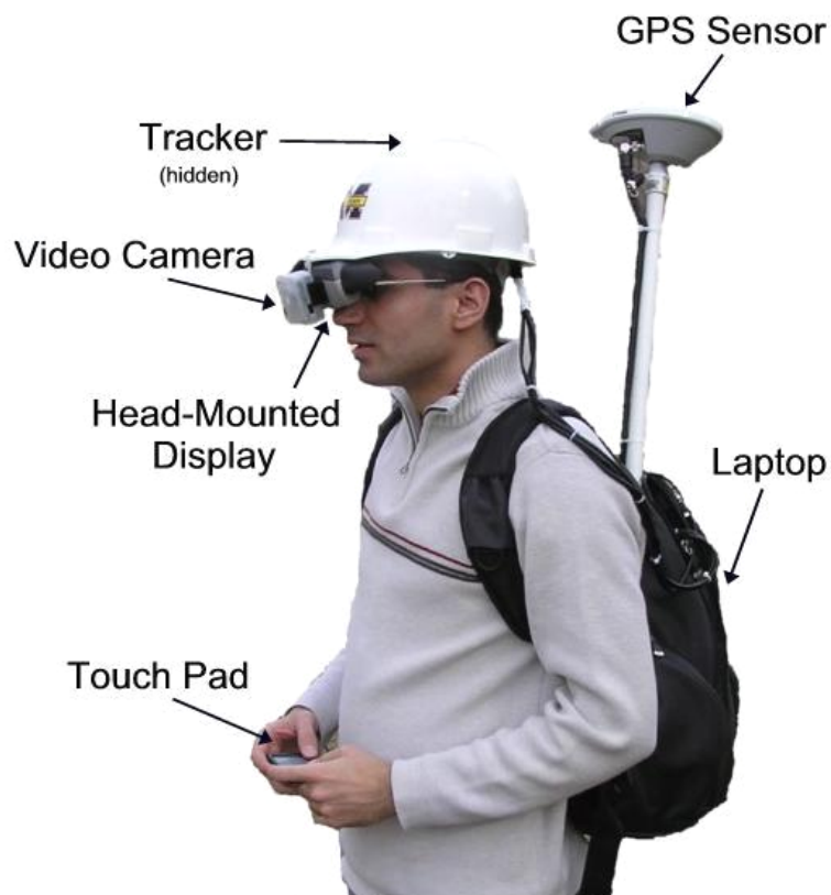
Figure 3.4 – Overview of the UM-AR-GPS-ROVER Hardware Framework
