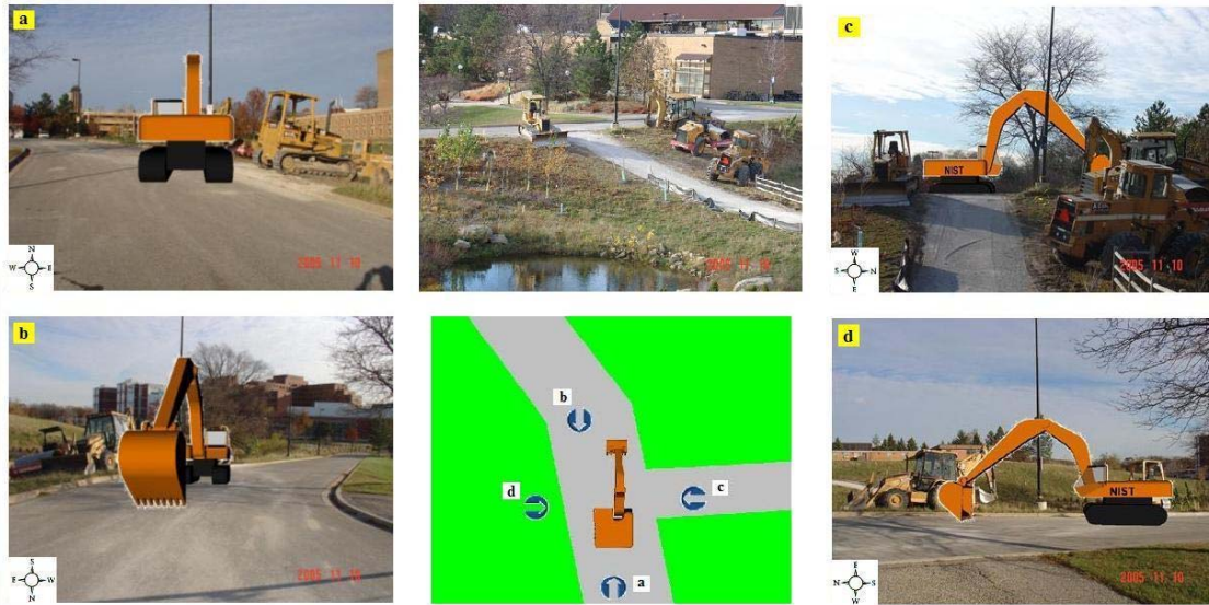
Figure 3.2 – Precise Registration of Virtual CAD Objects in an Augmented Scene
