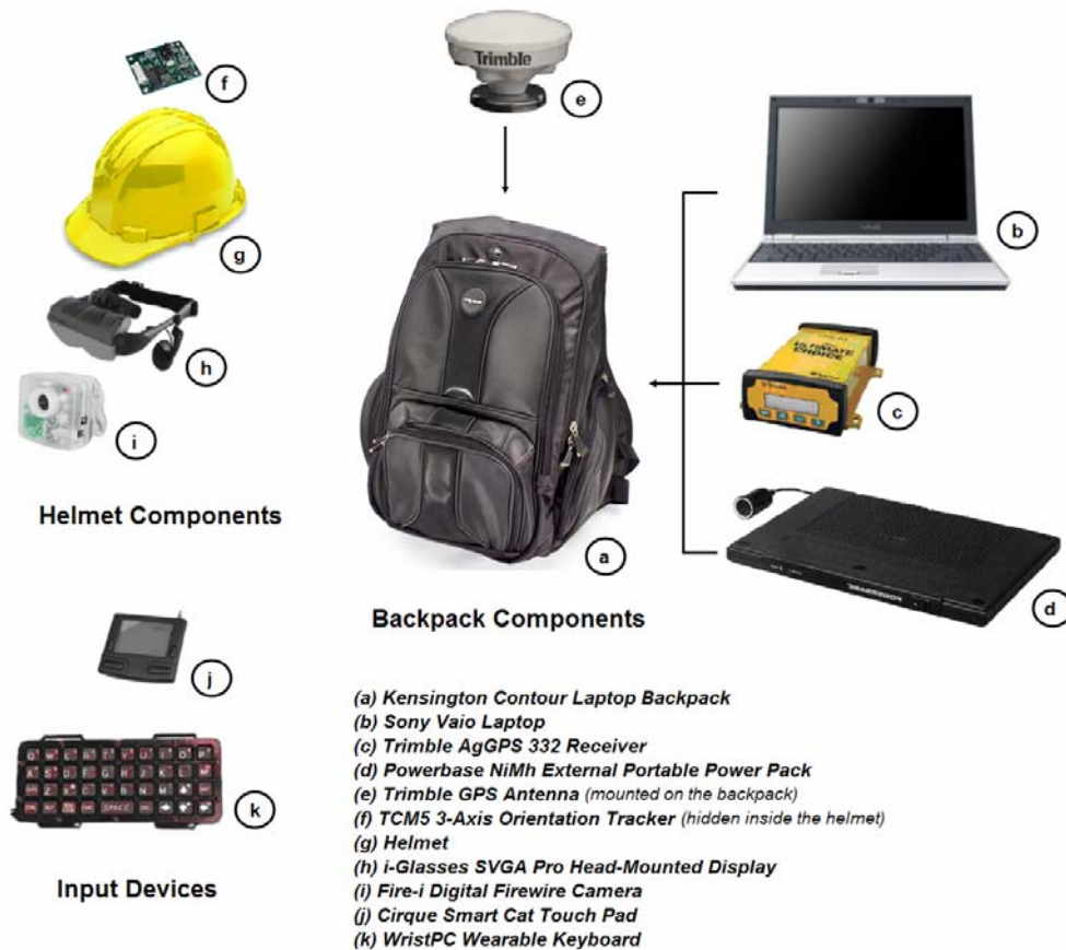
Figure 3.5 – Hardware Components of UM-AR-GPS-ROVER
