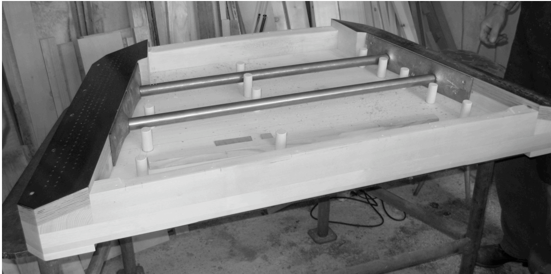
Figure 2.7. Interior of the cimbalom: oak soundboard and tuning-peg blocks, metal supporting frame, and soundposts.
