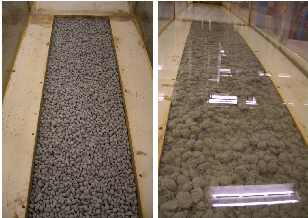
Figure 3.20: (a) AquaBlok ® bed before hydration, (b) AquaBlok ® bed under water after 21 hours of hydration.
