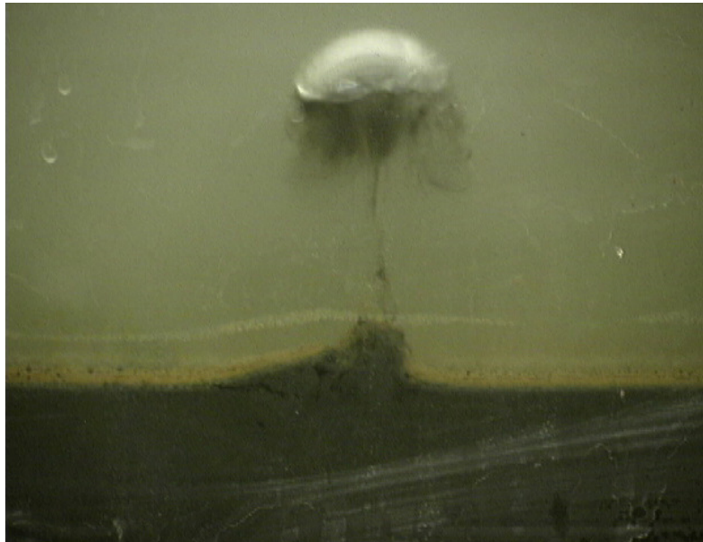
Figure 3.2c: Sediment is lifted up into the water column with the bubble.
