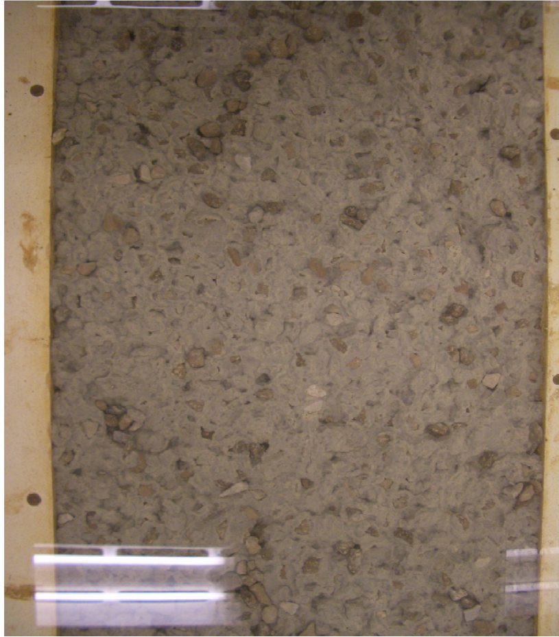
Figure 5.7: AquaBlok® bed surface after an experiment (aggregate adhering to the bentonite layer underneath creating an armor layer).
