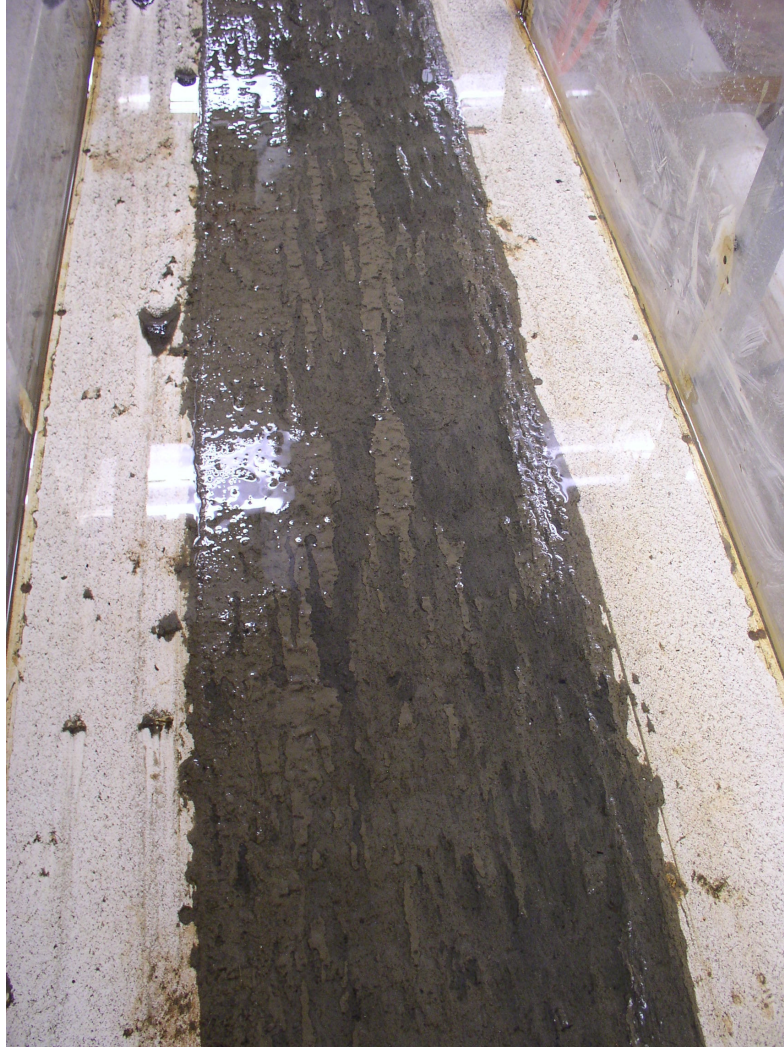
Figure 5.2: Eroded sediment bed surface with lighter colored oxidized sediment layer and the underlying darker layer at the eroded locations of the bed.
