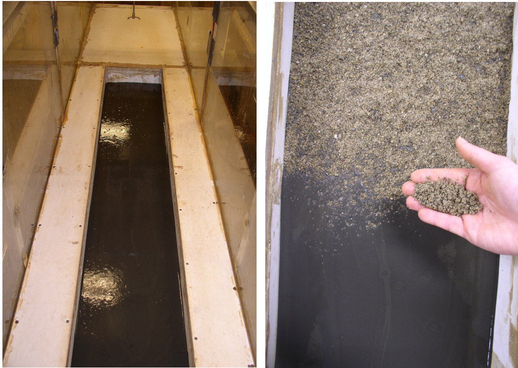
Figure 3.19: (a) The Anacostia River sediment placed in the cavity covering the soaker hoses right before placing the sand cap over it, (b) Careful placement of the sand cap over the sediment.
