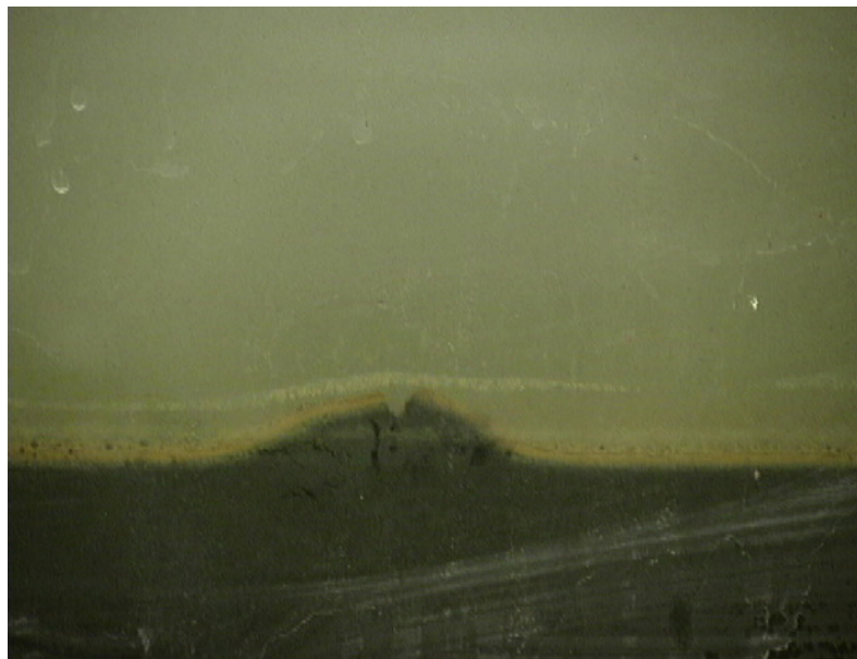
Figure 3.2a: Bulge development on the Anacostia River sediment surface just before the release of an air bubble.
