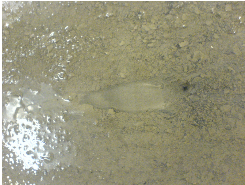
Figure 5.15: A view from the surface of a well-established channel formation in the cohesive sediment bed as a result of continuous air bubbling and local erosion created at close proximity of the channel (flow direction is from right to left and the channel is located towards the middle of the test section, the smooth surface is downstream from the bubble channel).
