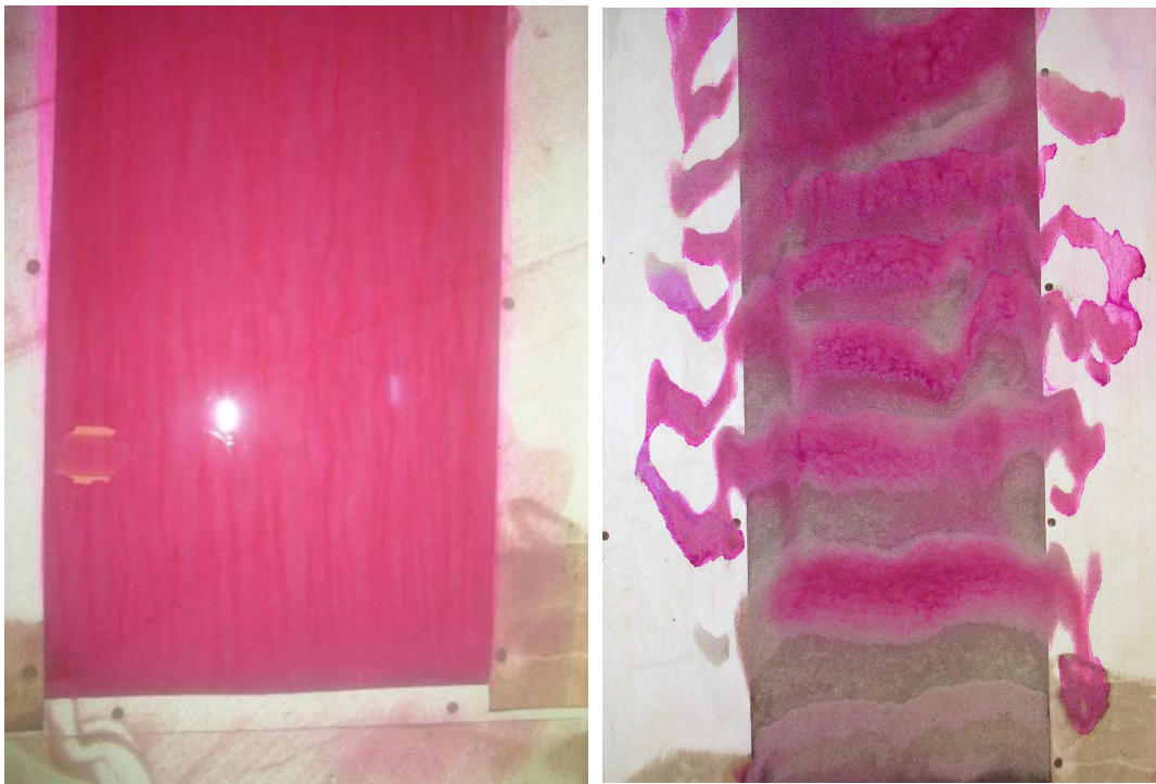
Figure 3.10: (a) Under a very low advective flow rate in the flume, the plan view of the test section after fluorescent dye was added to the injection system in order to test the uniformity of the seepage distribution over the whole bed, (b) Plan view of dyed ripple formations after application of a high flow rate over the bed (flow direction is from bottom to top of the photographs).
