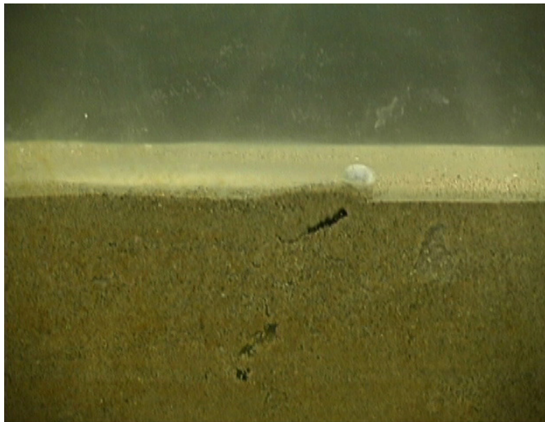
Figure 3.4: Channel formation and an air bubble along the side-wall of the tank (sand cap).
