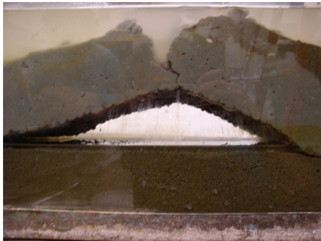
Figures 3.5: Evolution of the AquaBlok® - sand interface separation and subsequent cap failure due to air pressure build-up.
