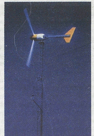
By locally generating electricity from the wind and sunlight, as well as collecting downed trees for wood, the couple have made their inn energy self-reliant. It's also fossil fuel free. A 10-kilowatt Bergey wind generator produces 7,000 to 9,000 kilowatt hours a year of electricity, more than meeting Inn Serendipity's needs.
