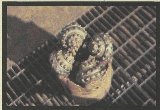
The four carbide-toothed cones of a roller core bit form a tool that looks like a sea anemone. Sediment rises up the hole in the middle of the bit's whirling cones into transparent tubes lining the core barrel.
